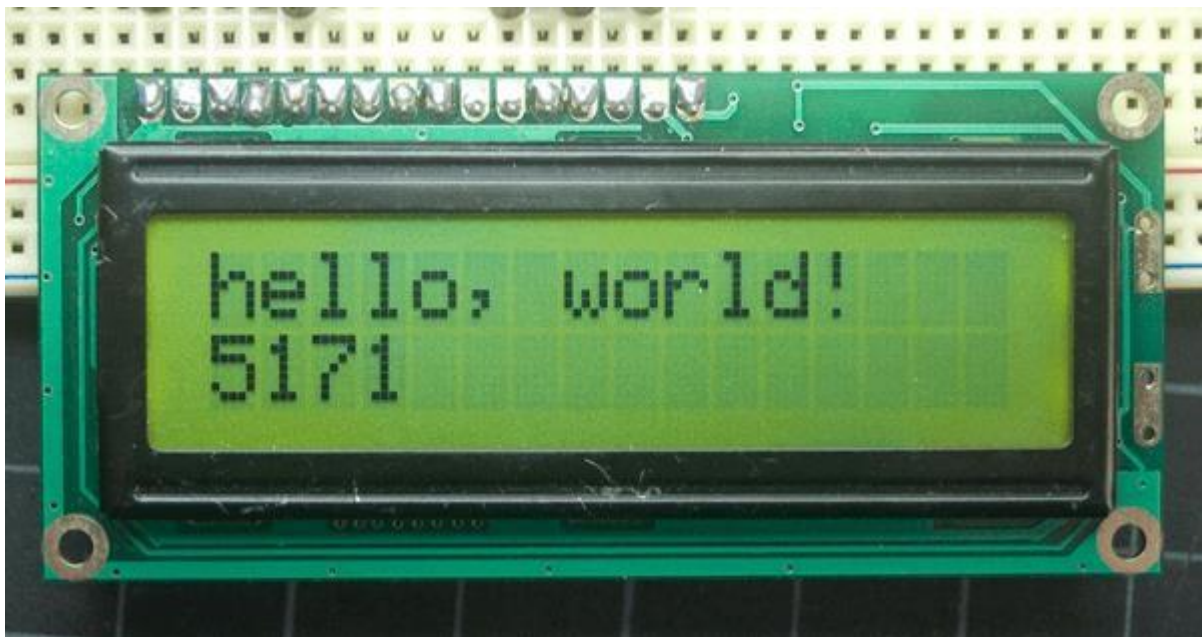
Fig. 21 Output of the sketch in 16x2 LCD
