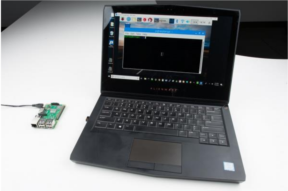
Fig. 10 Using RealVNC to access the Raspberry Pi's graphical desktop
